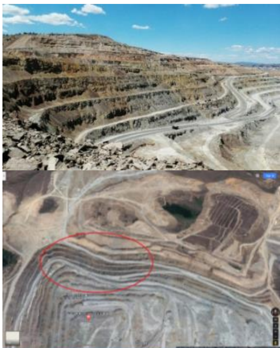
Figure 9. 2017.6 months - lateral slope, partial collapse / also soil 5 stack / and probable partial mine pressure
