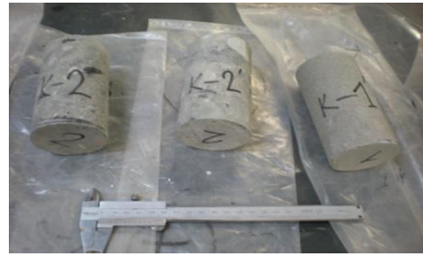
Fig.8. Samples preparation for laboratory tests
