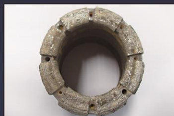
398m, HO PIE FACE DISCHARGE T3-B MEDIUM/ABRASIVE ROCK FORMATION NEVADA, USA
