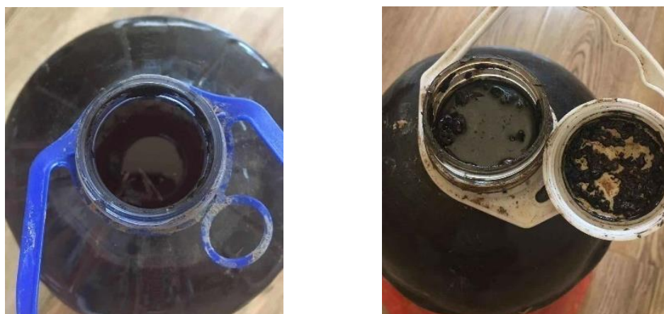
fig-2. Liquid samples from drilling waste
