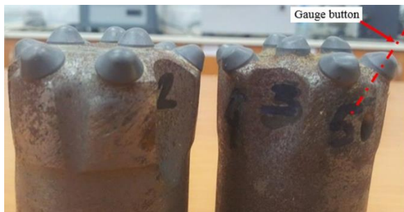
Figure 6. Gauge buttons of drill bits.
